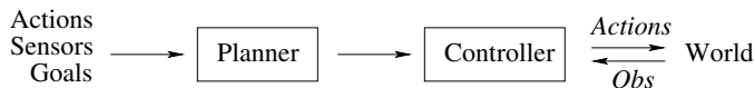
Figure 1. Planning is the model-based approach to autonomous behavior: a planner is a solver that accepts a compact model of the actions, sensors, and goals, and outputs a plan or controller that determines the action to do next given the observations.
